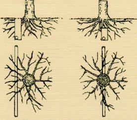
Less damage is done to tree roots if utilities are tunneled under a tree rather than across the roots.
