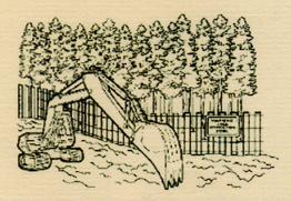
Protective fences should be erected as far out from the trunks as possible in order to protect the root system.
